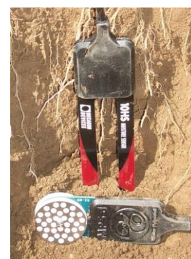
Figure 4. Sensors used to compare soil matric potential and volumetric measure volumetric soil moisture content. Photo taken on 15 June 2014.
