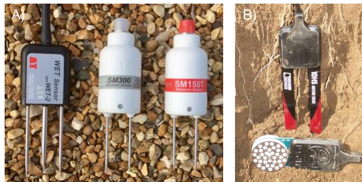
Figure GS2. A) Sensors used to measure volumetric soil moisture content, soil temperature and pore E.C. (Delta-T Devices Ltd). B) Sensors used to compare soil matric potential and volumetric soil moisture content (METER Group, Inc. USA).
