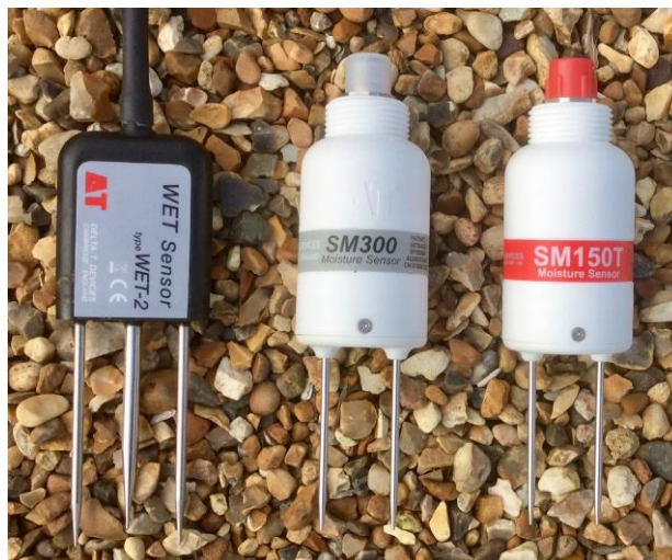
Figure 3. Sensors used to measure volumetric soil moisture content, soil temperature and pore E.C. Photo taken on 15 June 2017.
